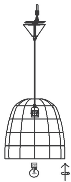
5. Insert the bulb by rotate
